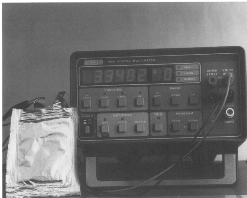
Fig. 2. Packaged polymeric lithium battery prototype.
